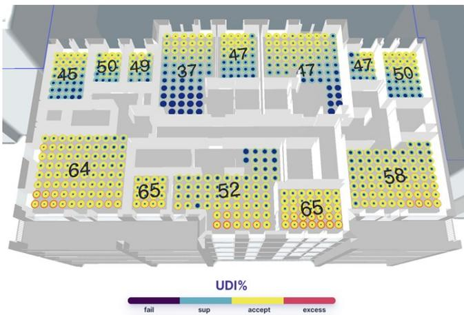
Figure 5. Application screenshot of daylight results in the converted model.
