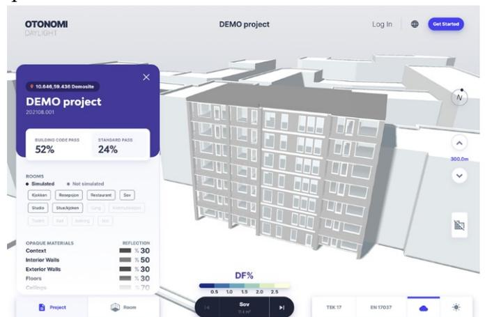
Figure 4. Application screenshot of a converted IFC model into a daylight model. Click to access.
